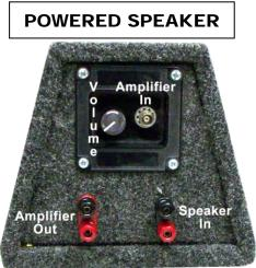
**2-17.** Check that the powered speaker volume is down. Reconnect the BNC to the Amplifier In of the powered speaker. Choose an instrument in Audio Quicktest, turn up the volume and listen to your amplifier. If you notice distortion it is because you are sending too much level to the amplifier. Turn down the output of the computer. You can also open Window Media Player and play some music from that Library.
