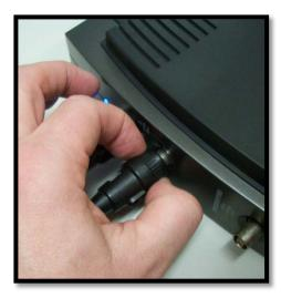
**2-16.** Now remove the BNC connector from the Oscilloscope interface Channel 2 by twisting the part closest to the interface to the left as shown to the left.
